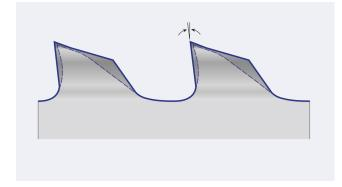
The PROFLEX® PREMIUM M42 is equipped with a special profile tooth form, which have a positive rake angle and a reinforced tooth back. The susceptibility
