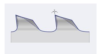
The special profile tooth features a positive cutting angle and reinforced tooth back edge. This reduces susceptibility to tooth breakage and vibration when sawing profiles.
