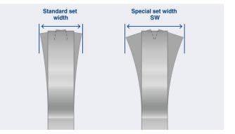
Standard set width compared to special set width SW: The extra wide set increases the free cut of the band saw blade so that there is more clearance to prevent jamming due to released material residual stress.
